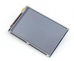
With the 3.5 Inch TFT Touchscreen-Display you can easily build a Mini-Tablet-PC based on an Raspberry Pi. The display, with a maximum resolution of 480x320 pixels, can be attached to the GPIO connections so that you won't need any mounting-skills.
