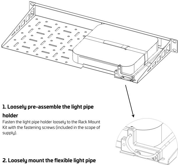
Fasten the light pipe loosely to the light pipe holder with the fixing screw(s) (included in the scope of supply).
